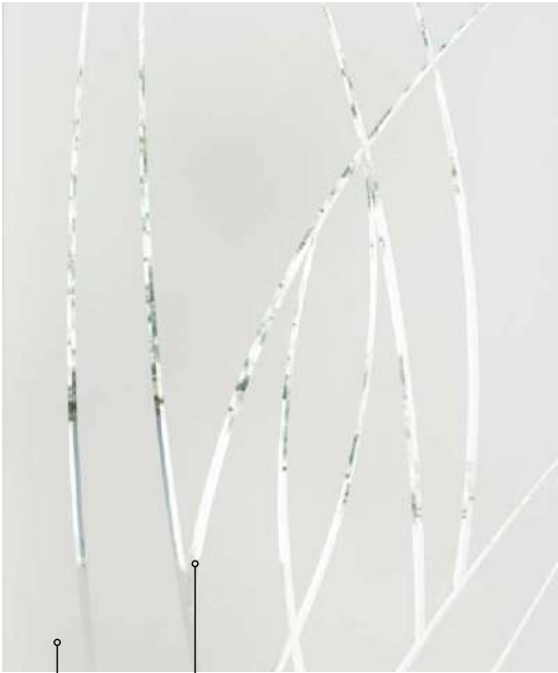
Sandblasted finish glass Polished V-Groove lines
